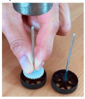
5. Push the axle holding the <u>gear wheel</u>, through the two brackets closest to the <u>two small</u> rectangular openings in the chassis. Use the bracket holes closest to the chassis.
