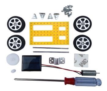
2. Screw the 4 small brackets to the chassis using the screws and screwdriver. Note that the longer <u>upright of the brackets are seated on the edge</u> of the chassis. Tip: Hold the bracket in position, then add the screws.
