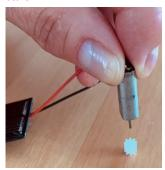
9. Install the motor: The motor is mounted closest to the large gear wheel. Use the second row of holes from the side – see photo. Screw the large motor bracket loosely to the chassis with four screws. Do not tighten yet. Handle wires with care. Then push the motor in so the teeth on the small gear wheel interlock with the large gear wheel. Check that the small gears do not touch the car wheel. Now, tighten the bracket screws.
